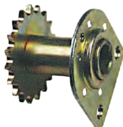
BEARING/SPROCKET Sprocket and bearing with standard for row unit. 19 tooth fits 7300 JD 7200 and 1700 series planters. Replaces JD no. AA35645. Hub width is 3.25"
