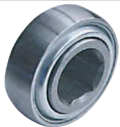
BEARING 7/8" hex bore. Has curved O.D. used on seed and fertilizer drives. Replaces JD no. AA22097.
